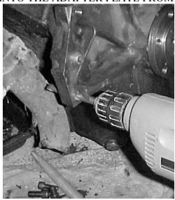
PLACE THE ADAPTER PLATE ONTO THE ENGINE BLOCK. IF NECESSARY USE A RUBBER MALLET TO FIT THE PLATE UP TO THE BLOCK FLUSH. DO NOT USE THE CAP SCREWS TO FORCE THE PLATE ONTO THE BLOCK. IF THE PLATE WILL NOT SIT FLUSH TO THE BLOCK, CHECK THE DOWEL PINS ON THE BLOCK. IF THEY PROTRUDE MORE THAN 3/8"OR HAVE BEEN DAMAGED AND THE ADAPTER PLATE IS FORCED ONTO THE BLOCK, THE ADAPTER PLATE WILL BE DAMAGED!
